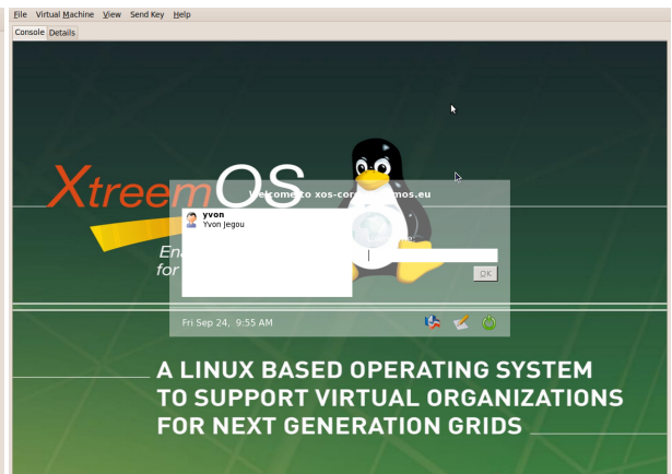
Figure 18: Installation is terminated, the installer has shut down. If the VM does not automatically reboot, it can be started from the manager window. After reboot, it is possible to log in as root or as the default user using this console.
